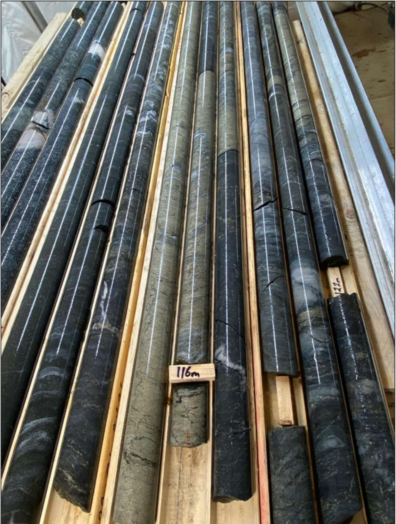
Figure 5 - Drill core from 2022 drilling at Ardiden's Dorothy prospect. Semi massive to massive sulphides present within a brecciated metavolcanic rock. Refer ADV ASX release 14 June 2022, 17 August 2022, and 26 September 2022.
