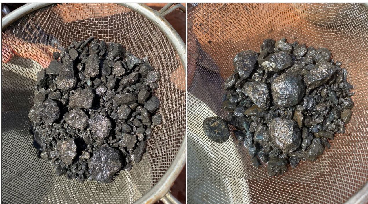
Figure 4: RC Drilling chips showing sulphide minerals from MMRC01 184-185m (left) and MMRC04 203-204m (right)
