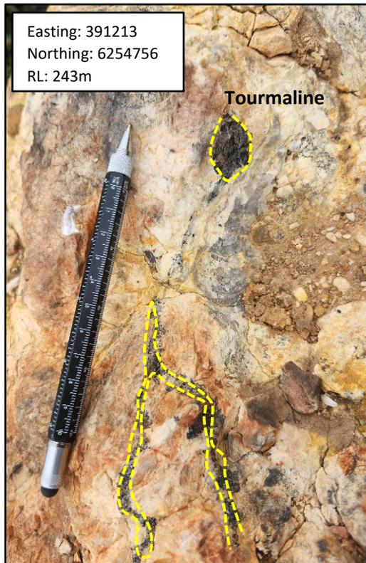
Figure 4: Sample RK000205. Pegmatite with coarse grained quartz, k-feldspar and tourmaline
