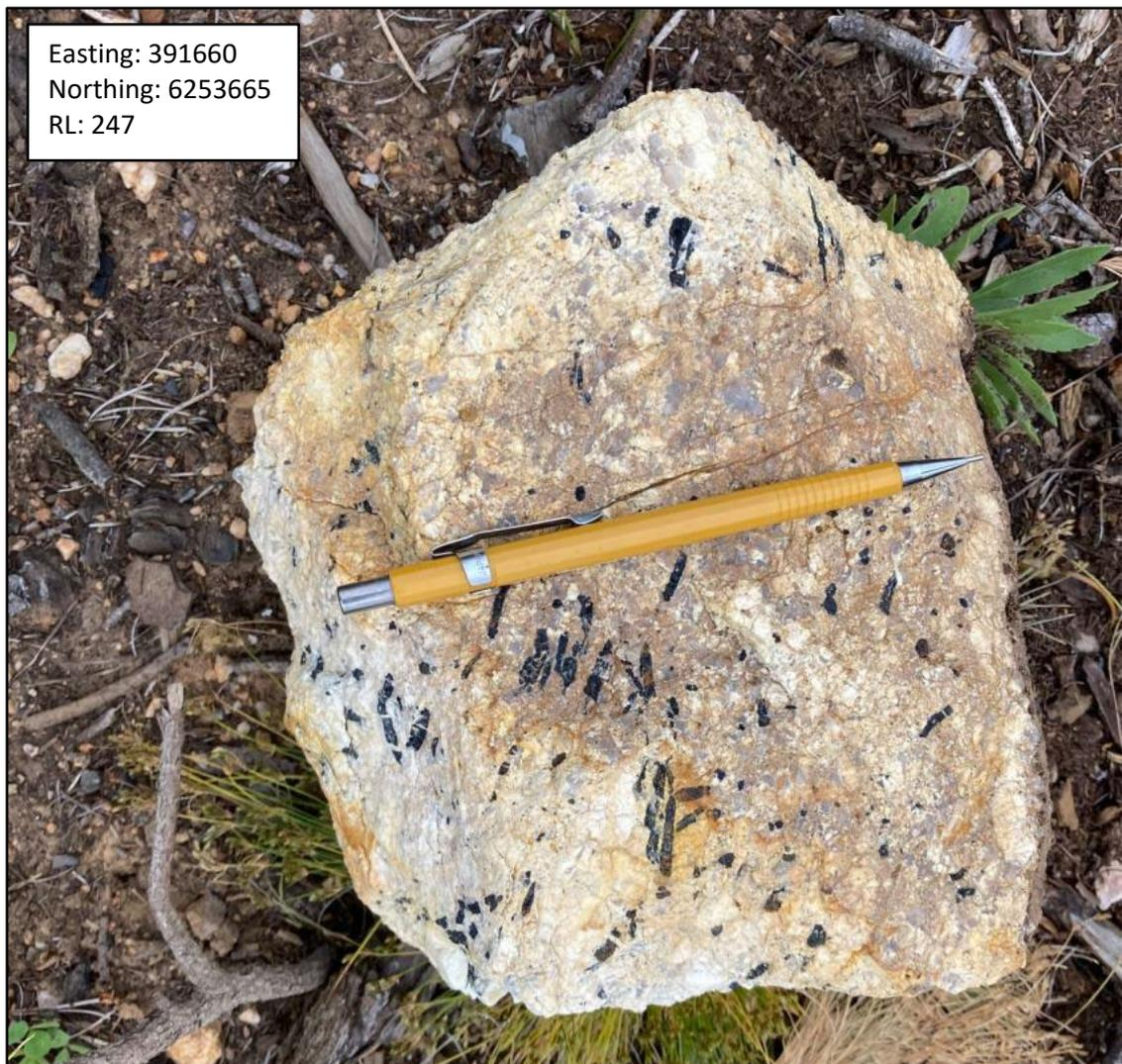
Figure 5: Sample RK000209. Pegmatite with coarse grained tourmaline
