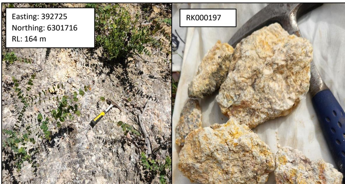
Figure 3. Sample RK000197. Weathered pegmatite with micas, quartz and potential relic spodumene.
