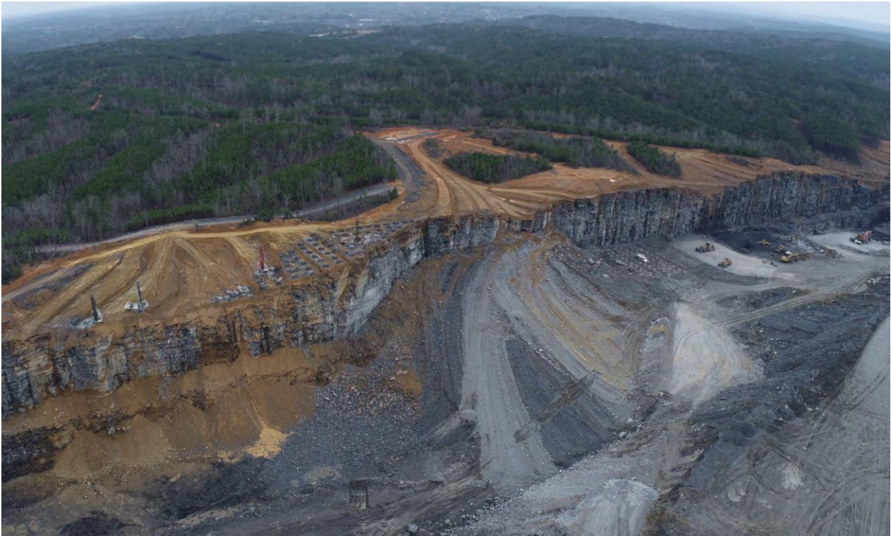
Image: Aerial shot of Black Warrior with dozer push paths visible in blasted ground
