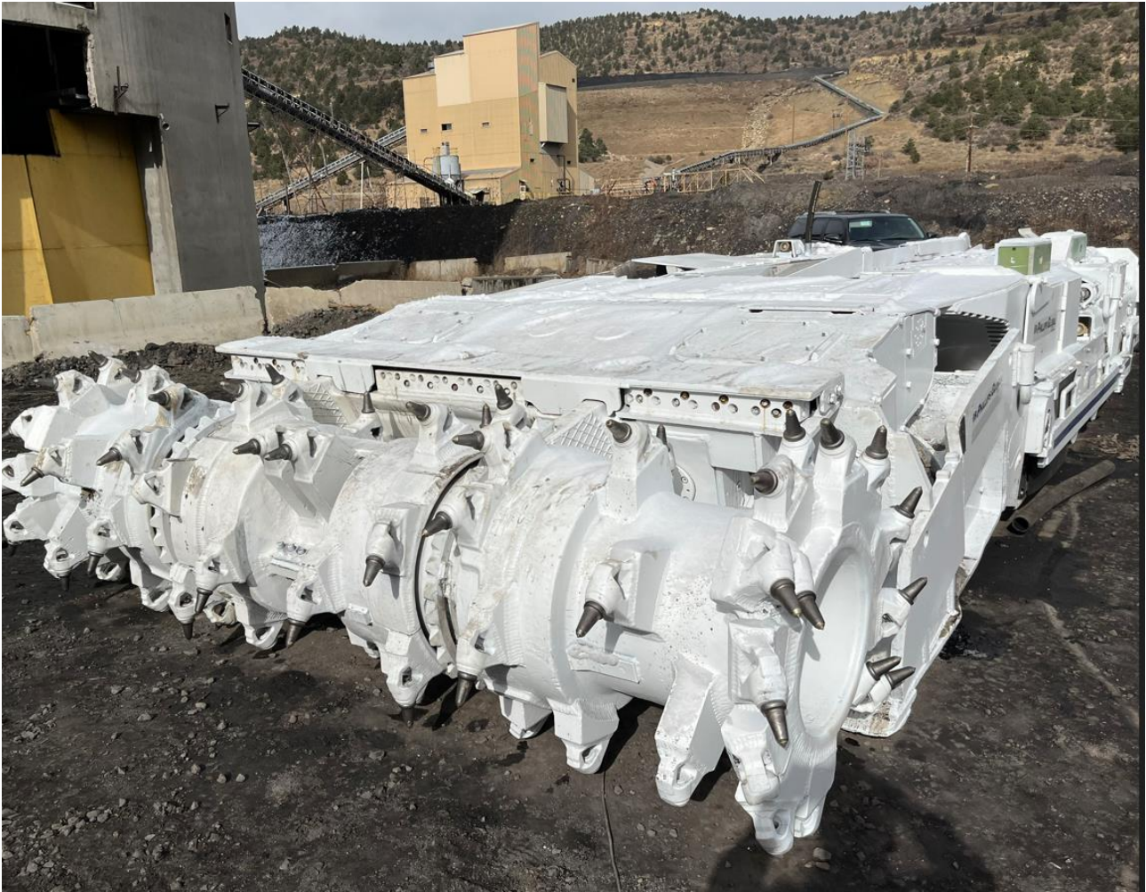
Image: CM04 at New Elk Mine – new cutterhead picks fitted and ready to be trammed underground
