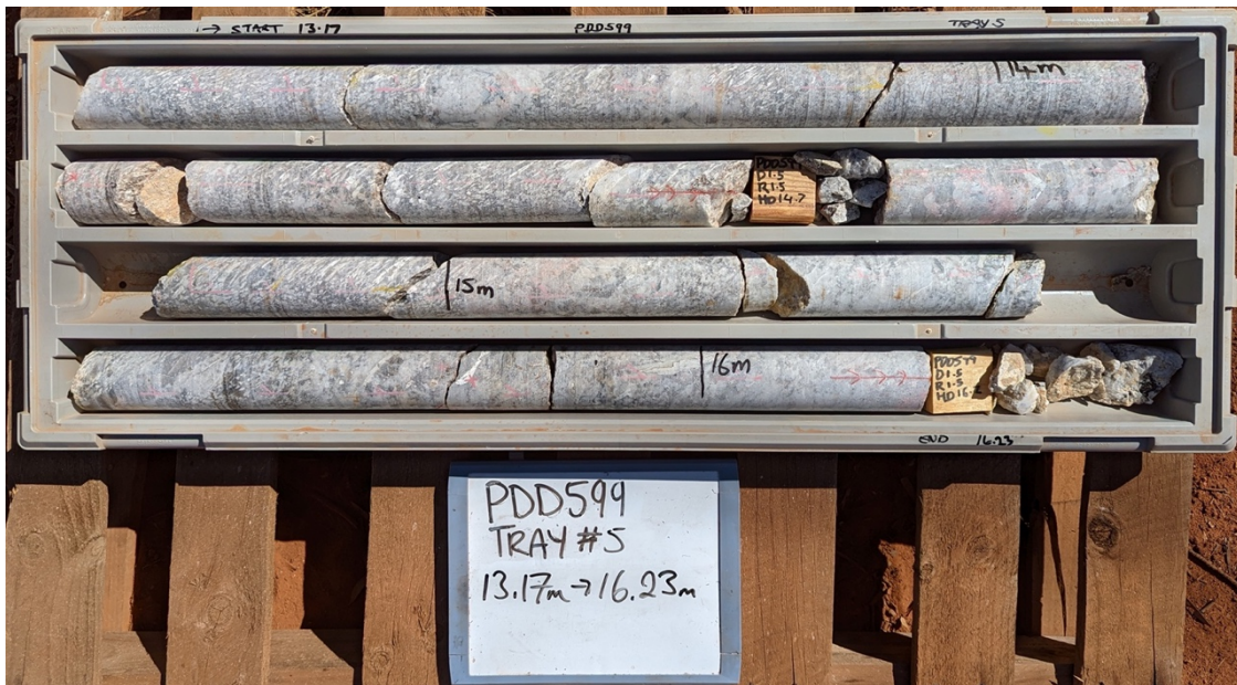
Figure 7 – Core photographs from PDD599 at Cade showing the strongly oxidised metasediments (host rock) against the relatively unweathered spodumene bearing pegmatite.
