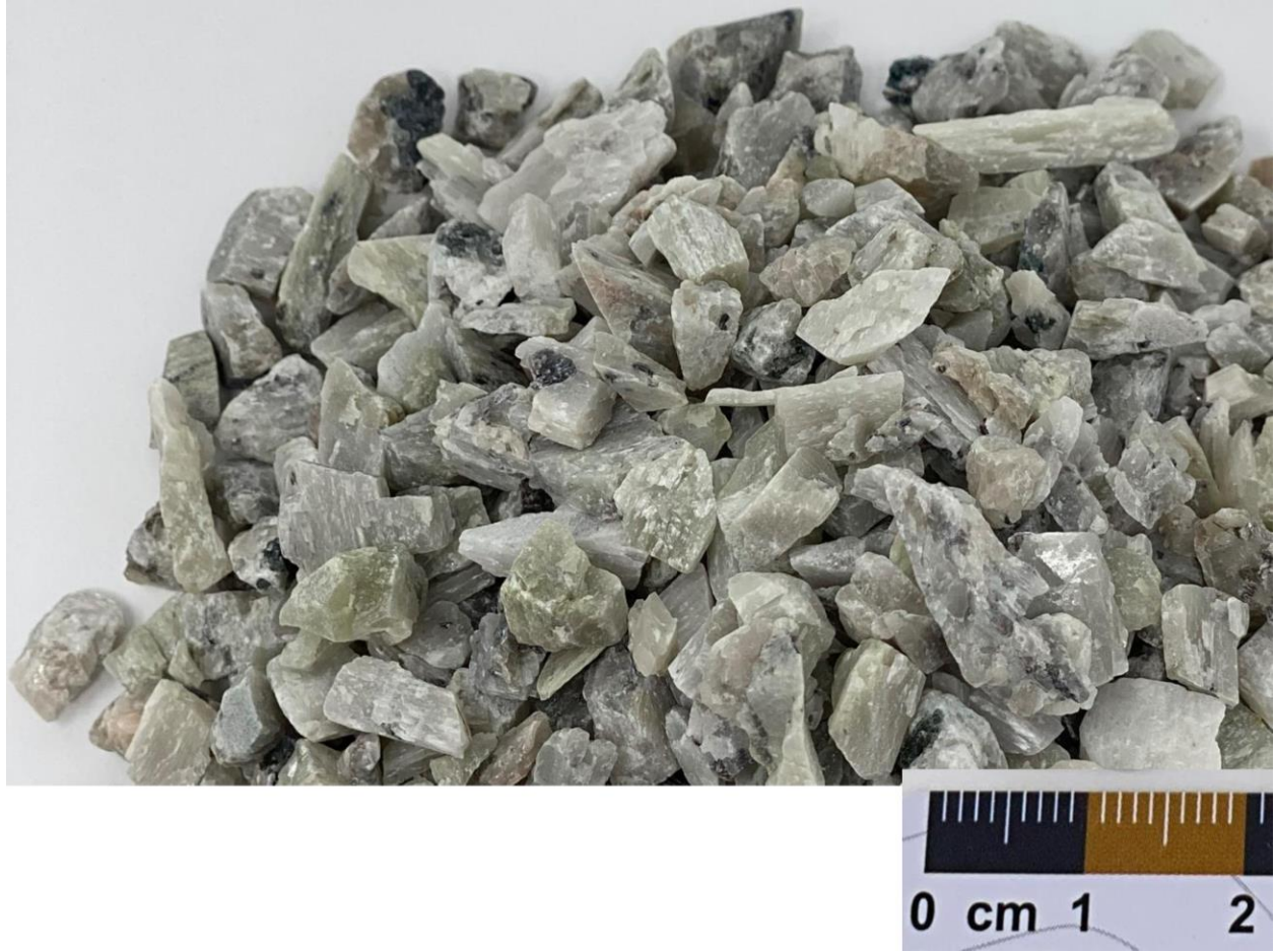
Figure 2: Close-up of spodumene concentrate (DMS + Non-Magnetic fractions) – 5.8% \text{Li}_2\text{O} and 0.60% \text{Fe}_2\text{O}_3 at 79% recovery
