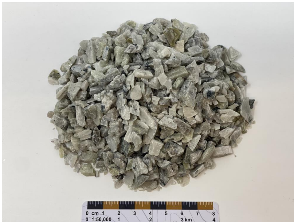
Figure 1: Spodumene concentrate (DMS + Non-Magnetic fractions) – 5.8% Li 2 O and 0.60% Fe 2 O 3 at 79% recovery
