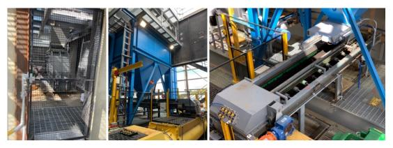
**Above**: hammer mill (left) sizes and screens the lignite before delivery to the surge hopper (centre). The weigh conveyor (right) controls the feed rate into the mixer (below left).
