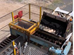
**Above**: Infeed system, where lignite is loaded and conveyed to the hammer mill.
