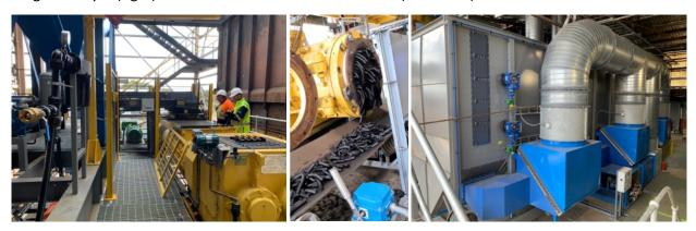
**Above**: the mixer adds a small amount of water to the incoming lignite to form a paste (left) before extrusion (centre). The extruded pellets are delivered to the conditioning system (right).
