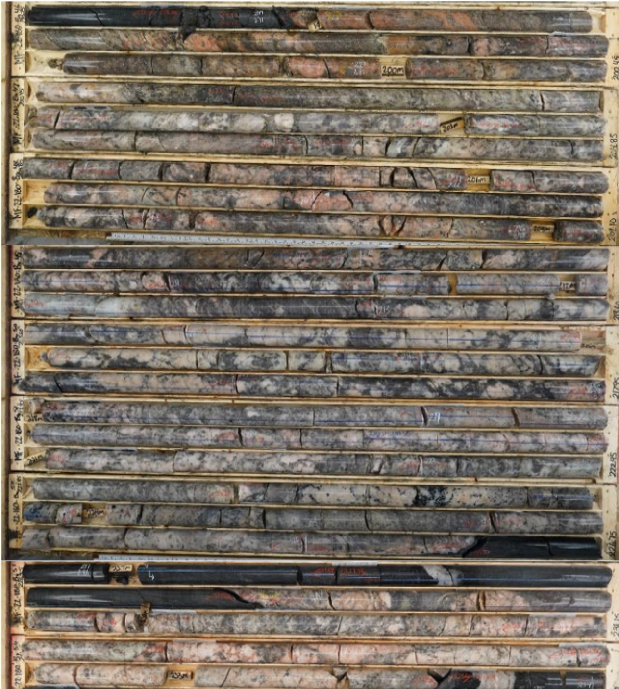
Figure 4 - MF22-180 drill core photo, over 30m of spodumene from 197m down hole
