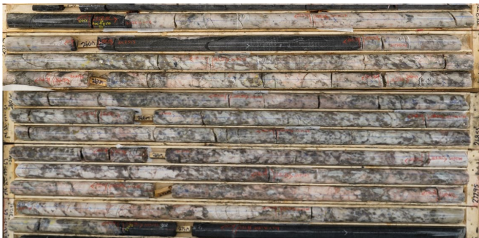
Figure 2 – MF22-177 drill core showing spodumene laths from 258.55 to 274.8m down hole, a potential new zone of spodumene mineralisation, stacked under the Mavis Lake Main Zone
