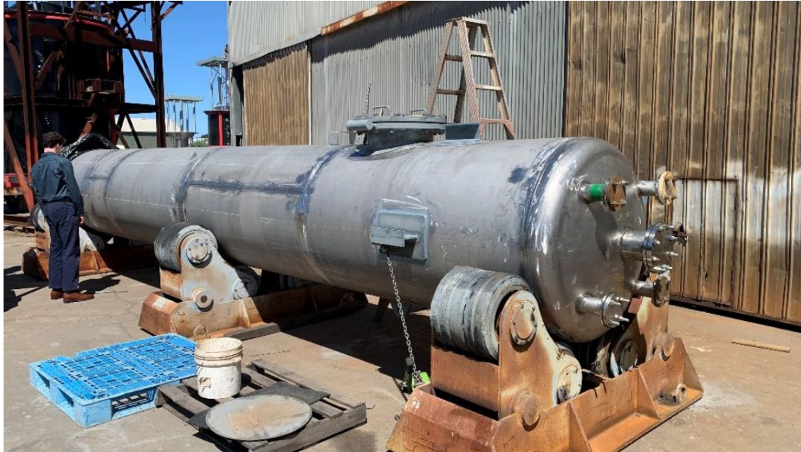
Figure 12: Elution column under hydrotest
