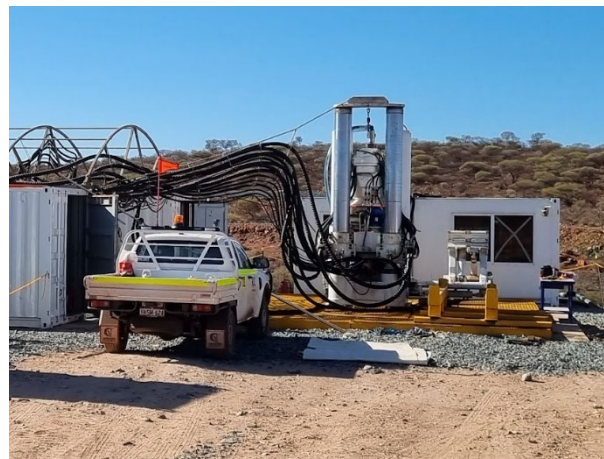
Figures 3-4: Left – Bellevue site RUC raisebore drilling at the Northern escapeway rise; Right – Second raisebore drilling rig at the Southern ventilation rise
