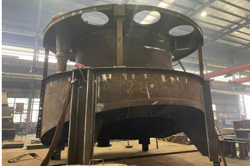
Figure 10: Cyclone cluster construction at factory
