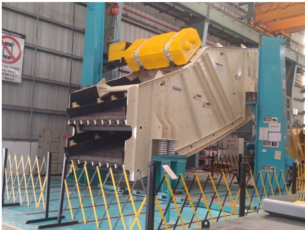
Figure 13: Crushing circuit screen testing
