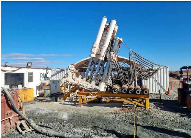
Figures 3-4: Left – Bellevue site RUC raisebore drilling at the Northern escapeway rise; Right – Second raisebore drilling rig at the Southern ventilation rise
