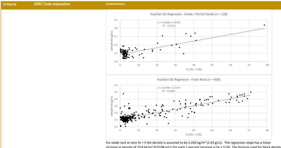
increase in density of 19.8 kg/m<sup>3</sup> (0.0198 g/cc) for each 1 percent increase in Fe + S (%). The formula used for block density (kg/m $^3$ ) determination in oxide rock is 2,430 + 19.8 x (Fe % + S%).
