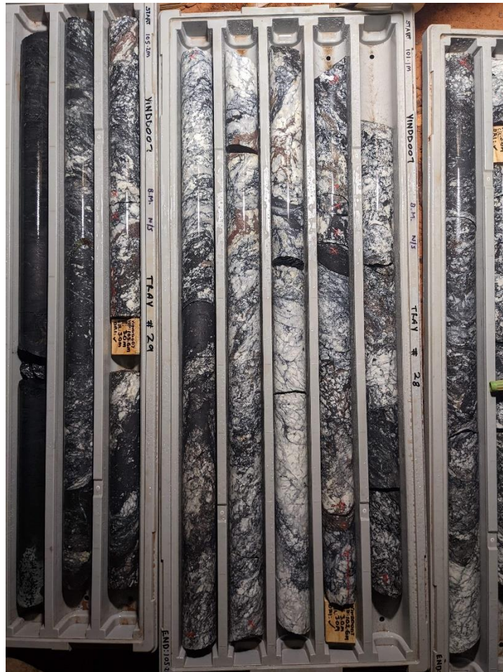
Figure 14: Photo of fresh ferrocarnatite from Yin hole YINDD007 ~100m to ~107m showing iron-magnesium carbonates (white), magnetite (black) and coarse monazite crystals (red).
