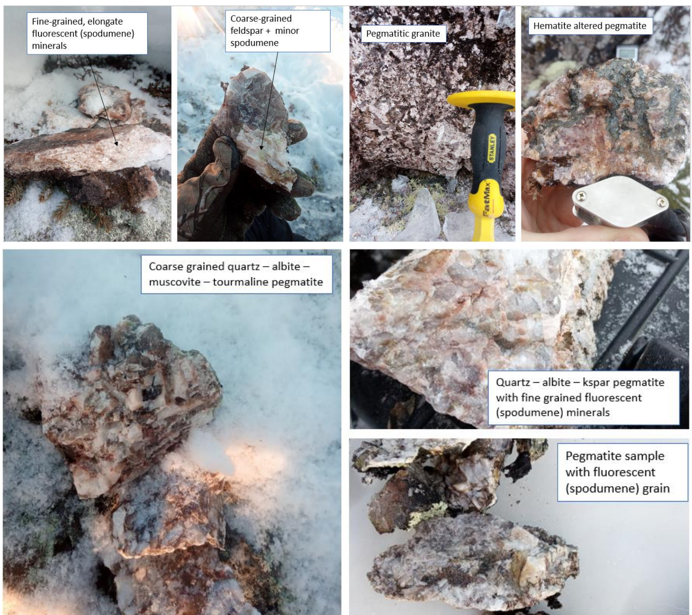
Figure 1: Various rock chip photos of pegmatite or pegmatitic samples taken during the field work program.
