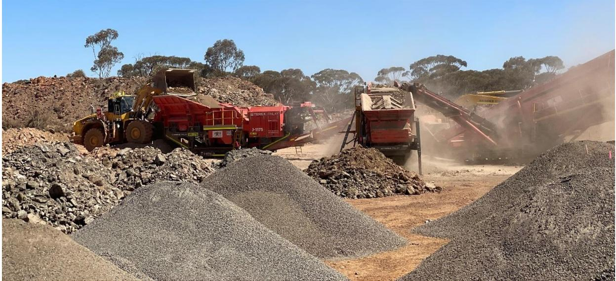
**Figure 1: Crushing operations at the 5A nickel mine, Spargoville W.A.**
