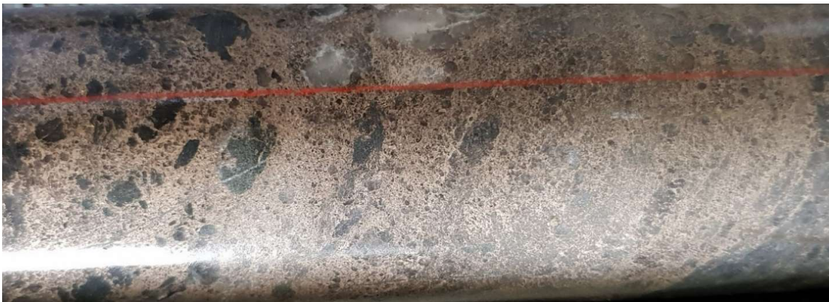
Image 1: Massive/breccia matrix sulphides in SBDD002 at 422.5m downhole, HQ core (results pending)
