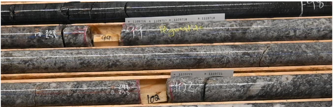
**Figure 3: RL-22-041 - Whole NQ diamond core showing high density spodumene crystal laths, 15.9m @ 1.12% Li<sub>2</sub>O from 98.1m (incl. 6.0m @ 1.91% Li<sub>2</sub>O from 99.0m)**
