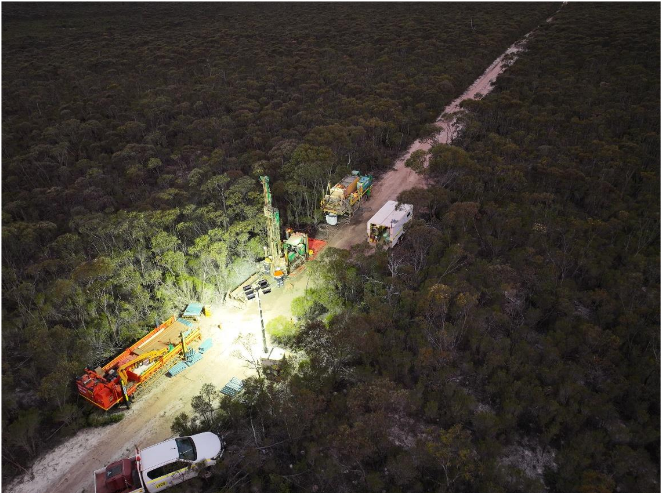
Photograph 1: 24 hours a day diamond core drilling yielded 961.5m of PQ core for metallurgical test work.
