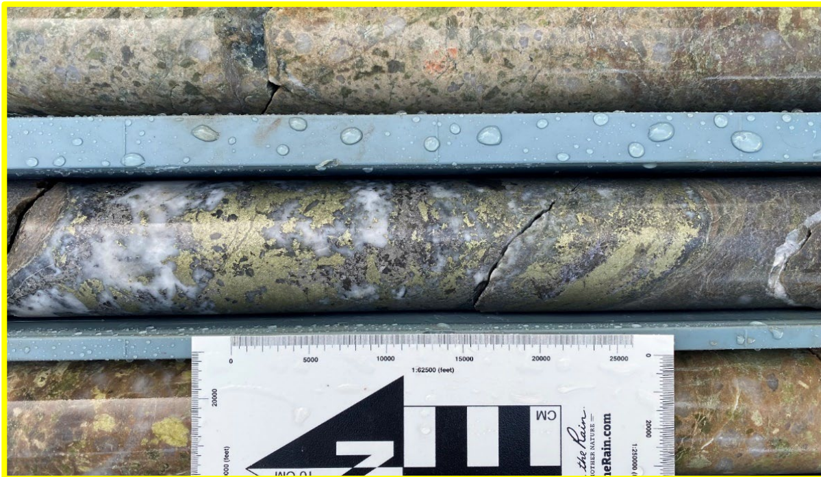
Figure 1 - Drill core photo of mineralised (chalcopyrite, galena, arsenopyrite, pyrite) veining in altered granite porphyry, and close up of significant copper intercept 1m @ 3% Cu from 173m (22NGD108).
