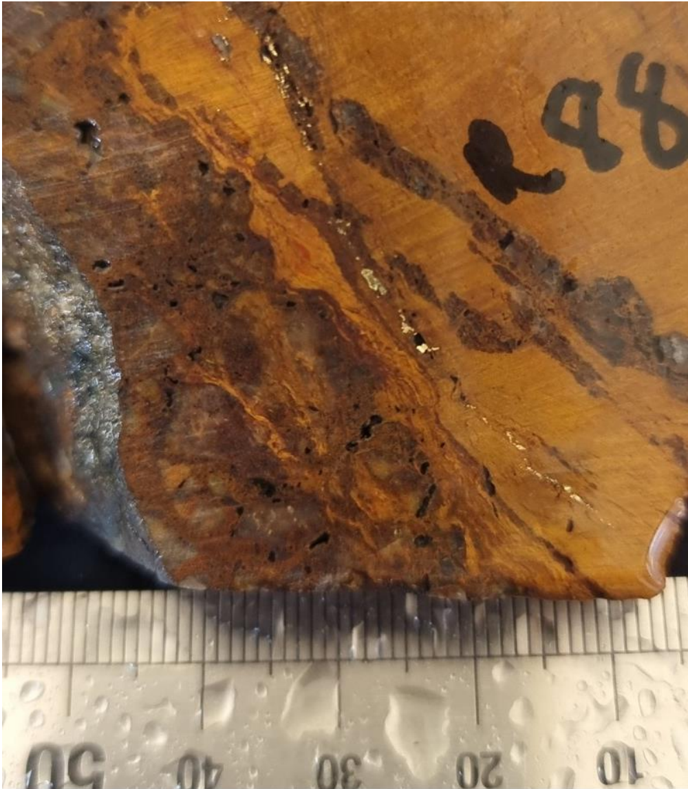
Figure 2: Core C close up showing gold vein
