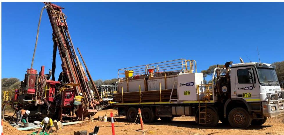
Figure 1: Photo of the RC drill rig on site at Windinne well.
