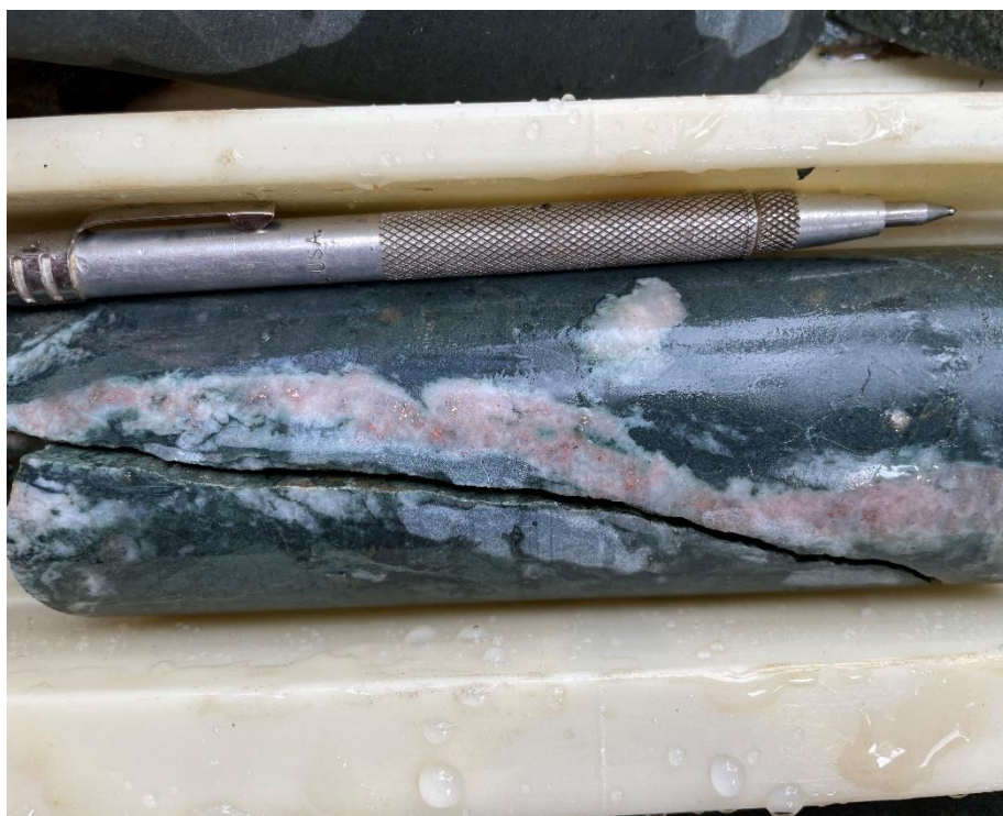
Figure 2. 22RRD-03 159.20m-160.80m depth contains dense silica+carbonate veins, up to 1-3% native copper
