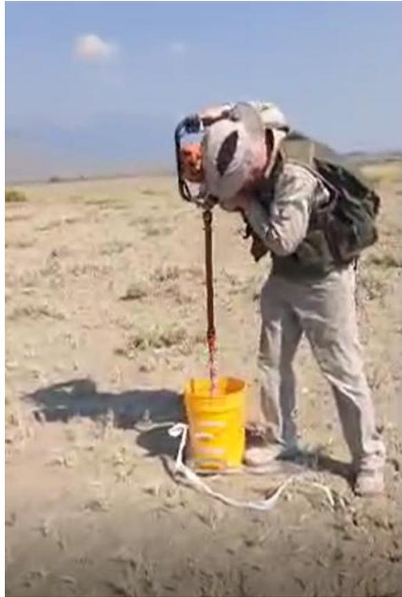
Figure 3: Auger Sampling
