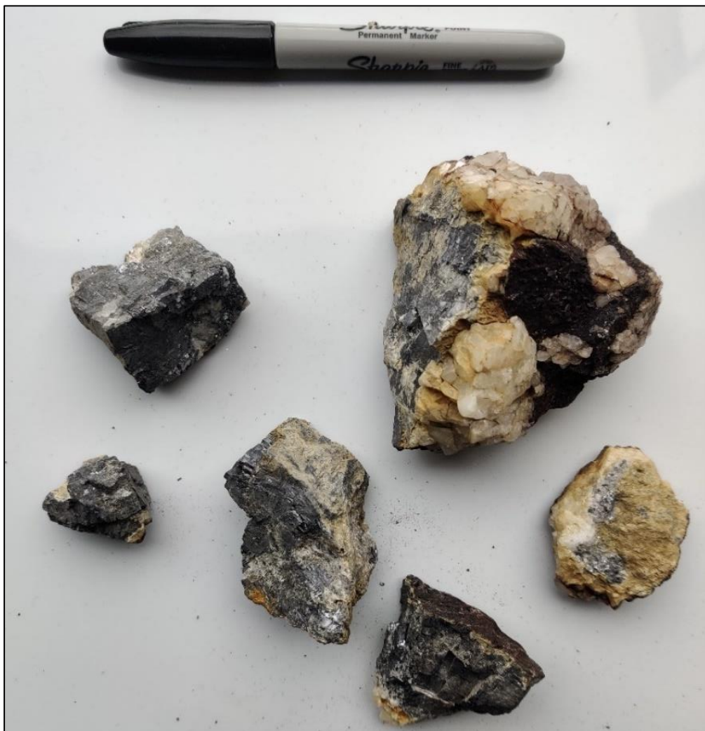
Figure 8. Nuldal rock chip sample 9959. Quartz vein-hosted massive galena, containing 183 g/t Ag and 21.6% Pb.
