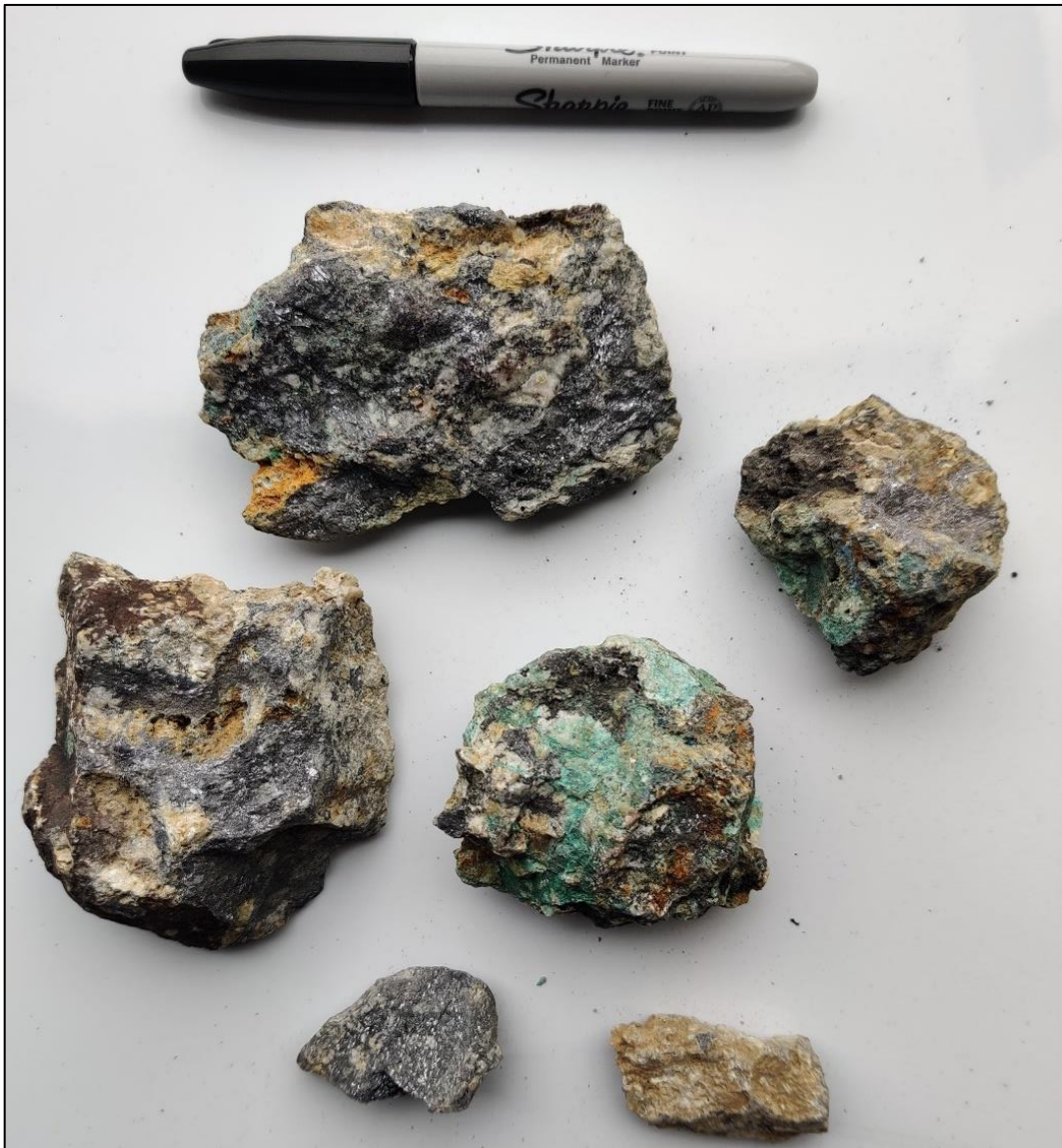
Figure 11. Holberg rock chip sample 9963. Quartz vein-hosted massive galena and malachite, containing 76 g/t Ag, 18.98% Pb and 0.44% Cu.
