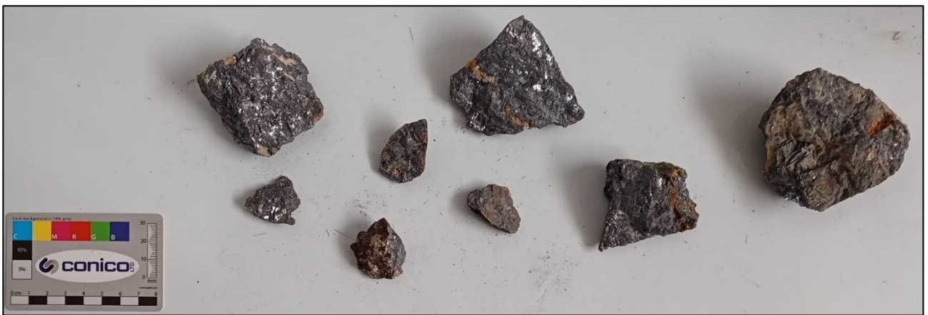
Figure 12. Sortebjerg rock chip sample 9970, consisting of quartz vein-hosted massive galena, containing 226 g/t Ag, 0.15% Cu and 22.5% Pb.
