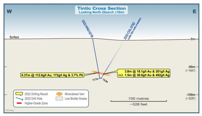
Figure 2 – Tintic interpreted drill cross section (diamond hole 2022-KNG-021B and RC hole CHL-075D)
