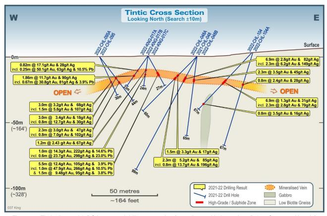
Figure 1 – Tintic diamond & RC interpreted drill cross section (note diamond holes 17A, 17B & 17C reported herein)
