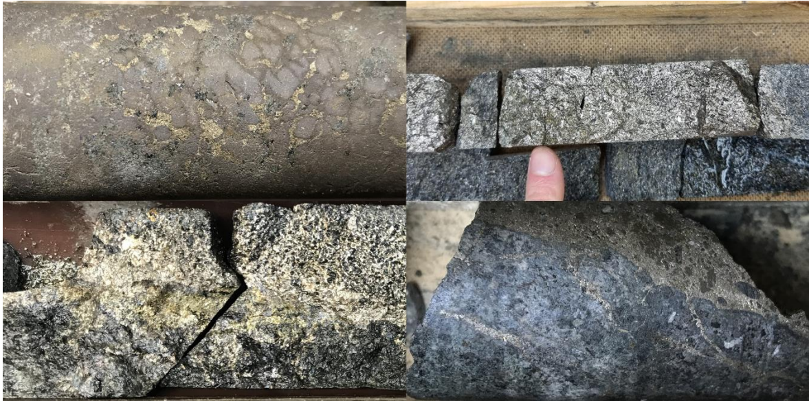
Figure 6: Historic drill core photos. Top left: massive pyrrhotite-pentlandite with pentlandite occurring as coarse loops (Bruvann BH-265-125, 1m @ 3.08 % Ni); Top right: massive pyrrhotite-pentlandite (Rånbogen SH-004, 0.35m @ 2.52 % NiS); Bottom left: net-textured sulphides in poikilitic harzburgite cross-cut by soft-walled sulphide vein (Bruvann, DH1061-01, 2m @ 0.7% Ni); Bottom right: massive sulphide vein breccia cutting olivine pyroxenite (Bruvann, BH-265-125, 1.25m @ 1.6 % Ni).
