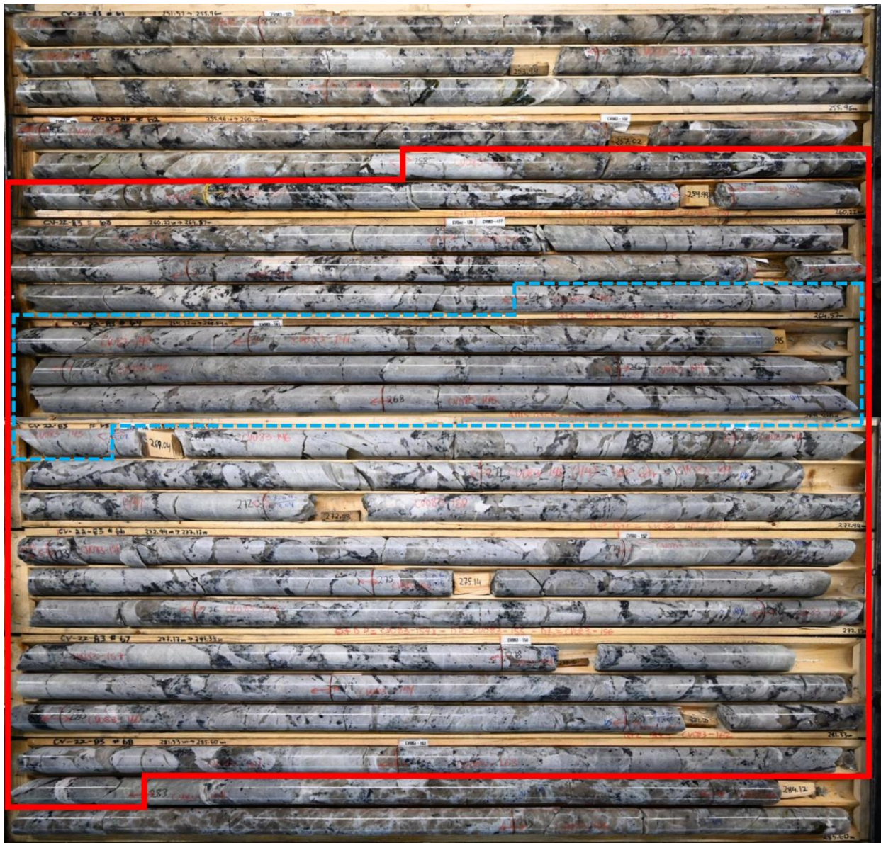
Figure 2: High-grade drill core intersection (25.0 m at 5.04% \text{Li}_2\text{O} ) in CV22-083 (red box), including 5.0 m at 6.36% \text{Li}_2\text{O} (dashed blue box)
