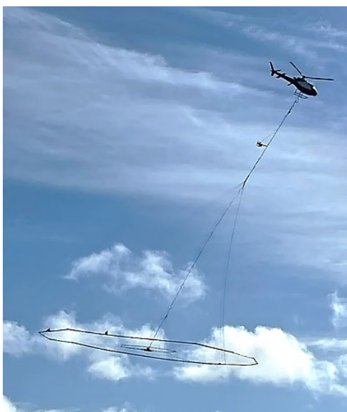
Figure 2: VT MAX and transmitter and receiver array and magnetometer during a helicopter borne survey .
