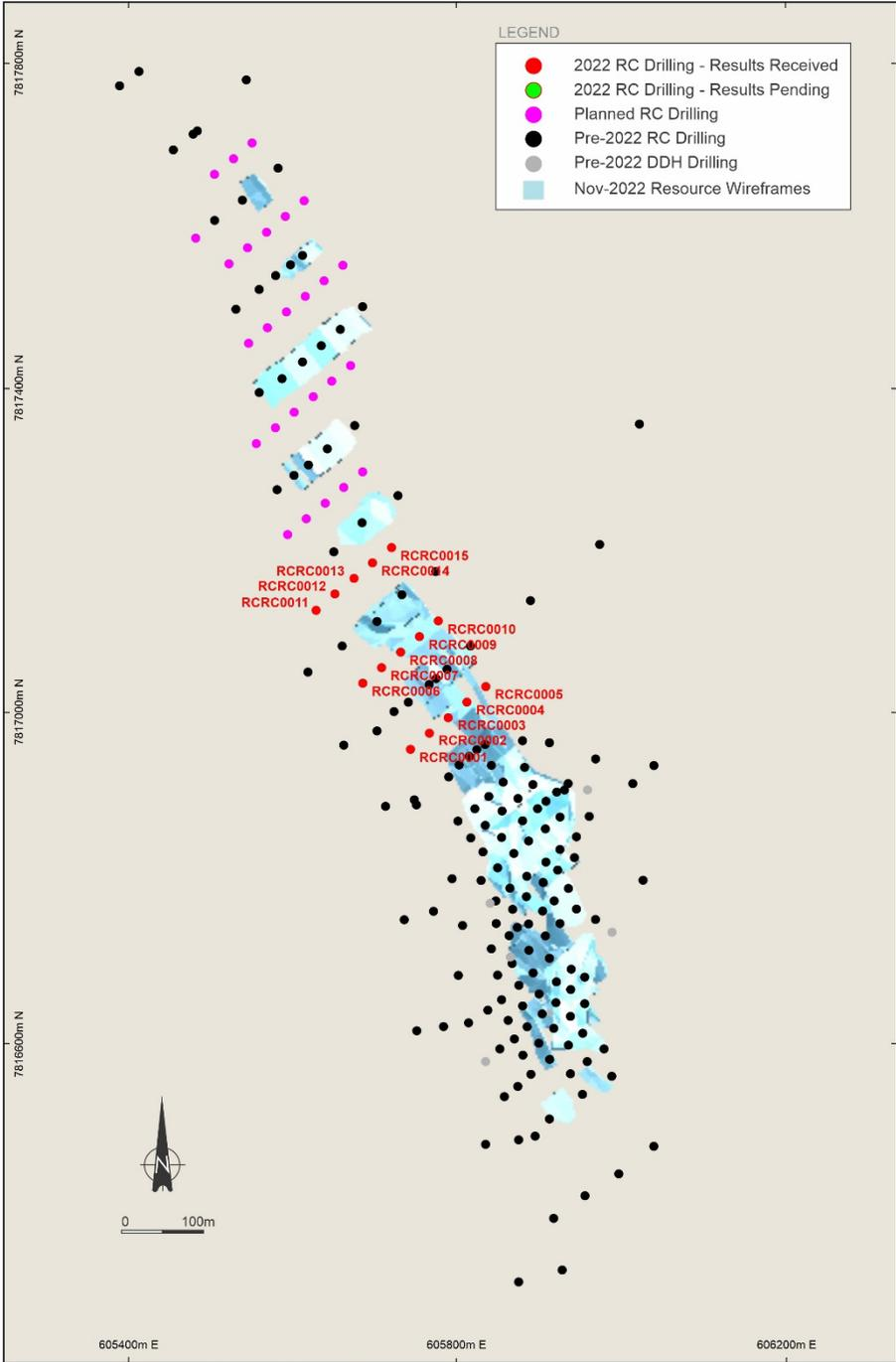
Figure 2 – Plan view of the Ripcord area displaying location of drilled and planned drill hole collars
