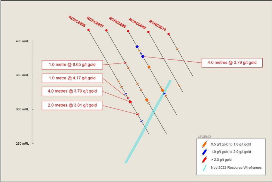
Figure 4 – Drill Hole Cross Section RCRC0006 to RCRC0010.
