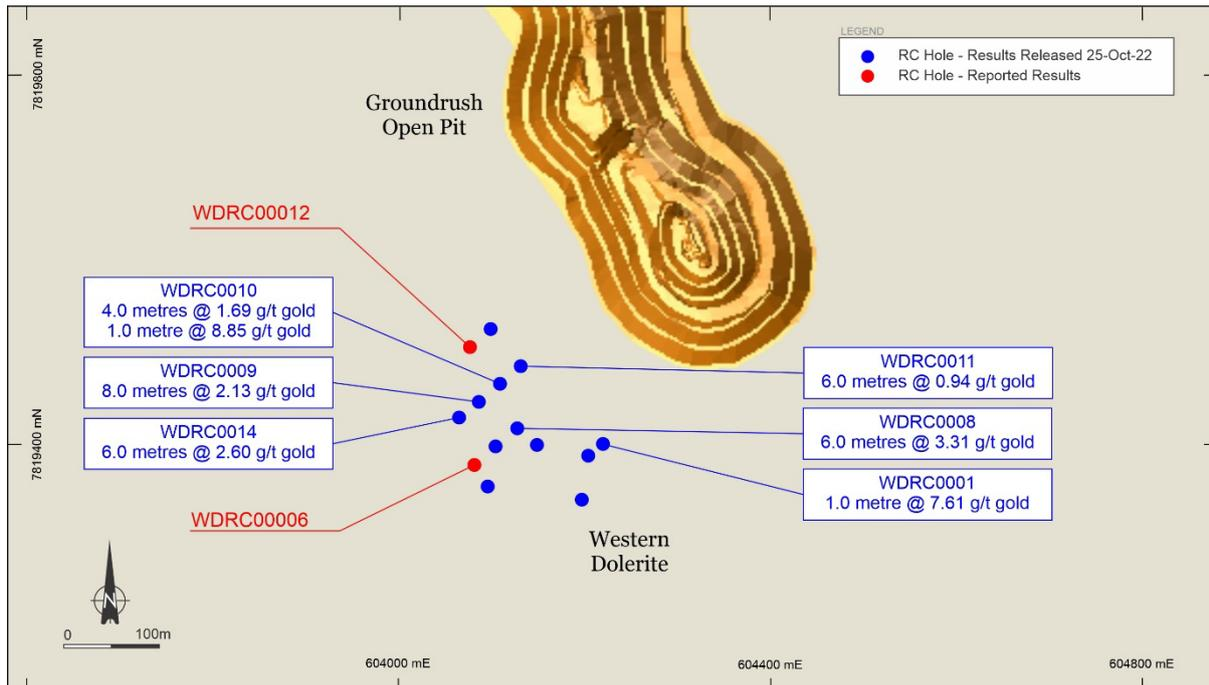
**Figure 6 – Plan view of the RC drill campaign completed at the Western Dolerite Prospect. Displayed results previously reported to the ASX on the 25 October 2022 – Update on Recent Drilling Activities Completed on the Central Tanami Project.**
