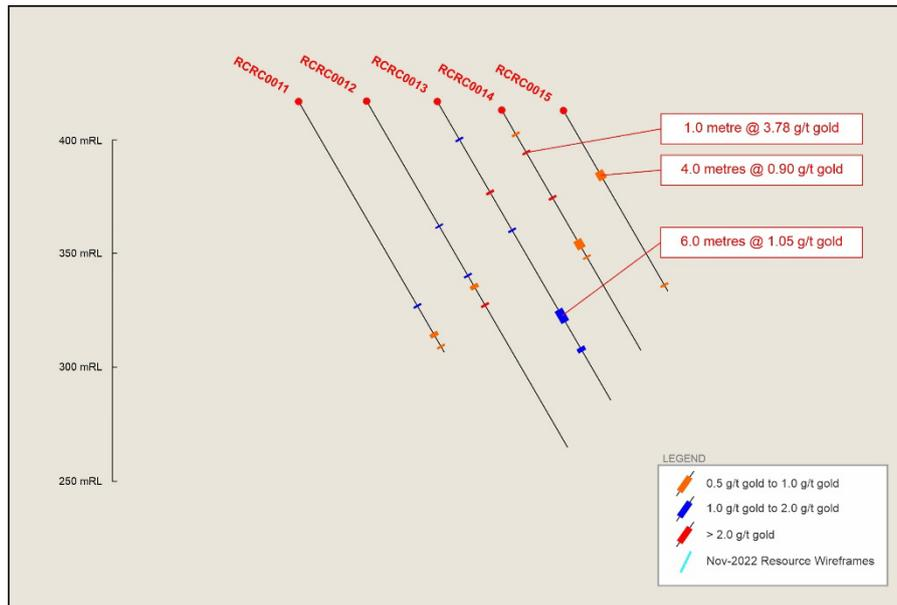
Figure 5 – Drill Hole Cross Section RCRC0011 to RCRC0015.
