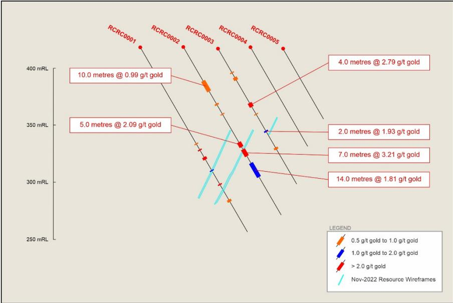
Figure 3 – Drill Hole Cross Section RCRC0001 to RCRC0005.
