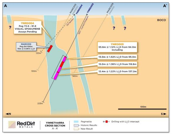
Figure 1: Cross Section showing YNRD005.
