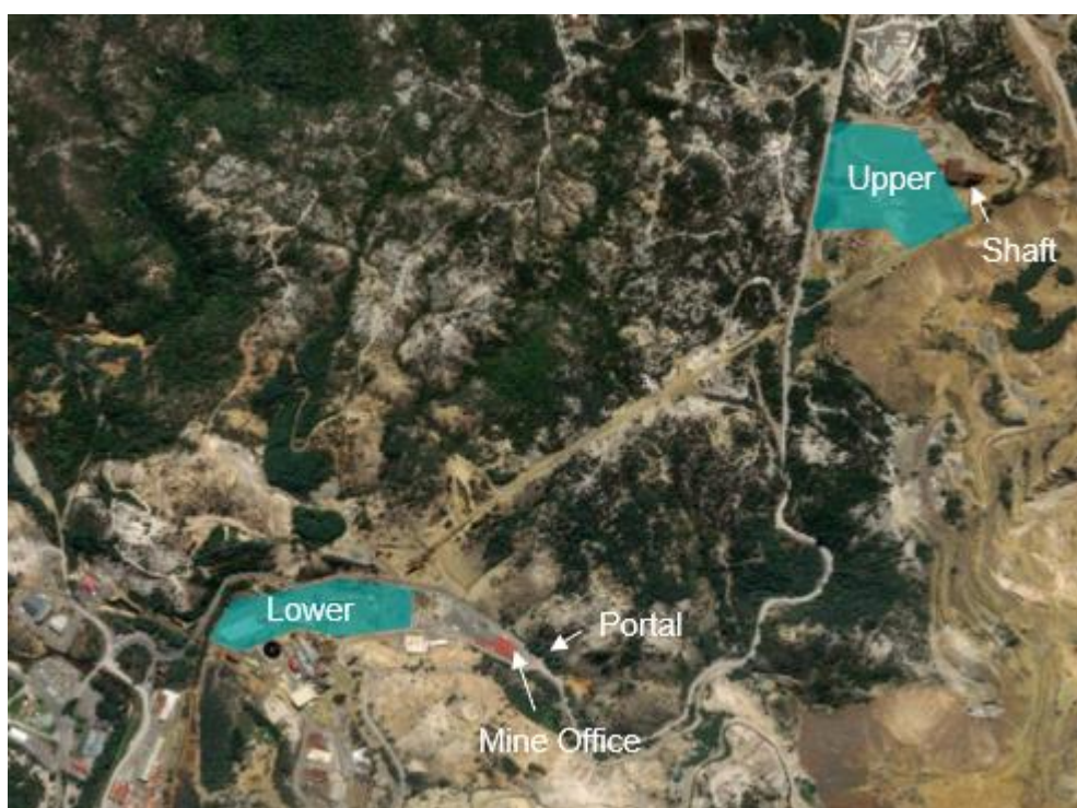
Figure 22 – Process plant location options
