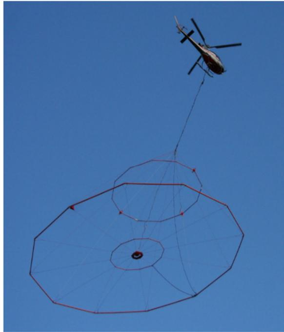
Figure 3: Helicopter with VTEM receiver underneath
