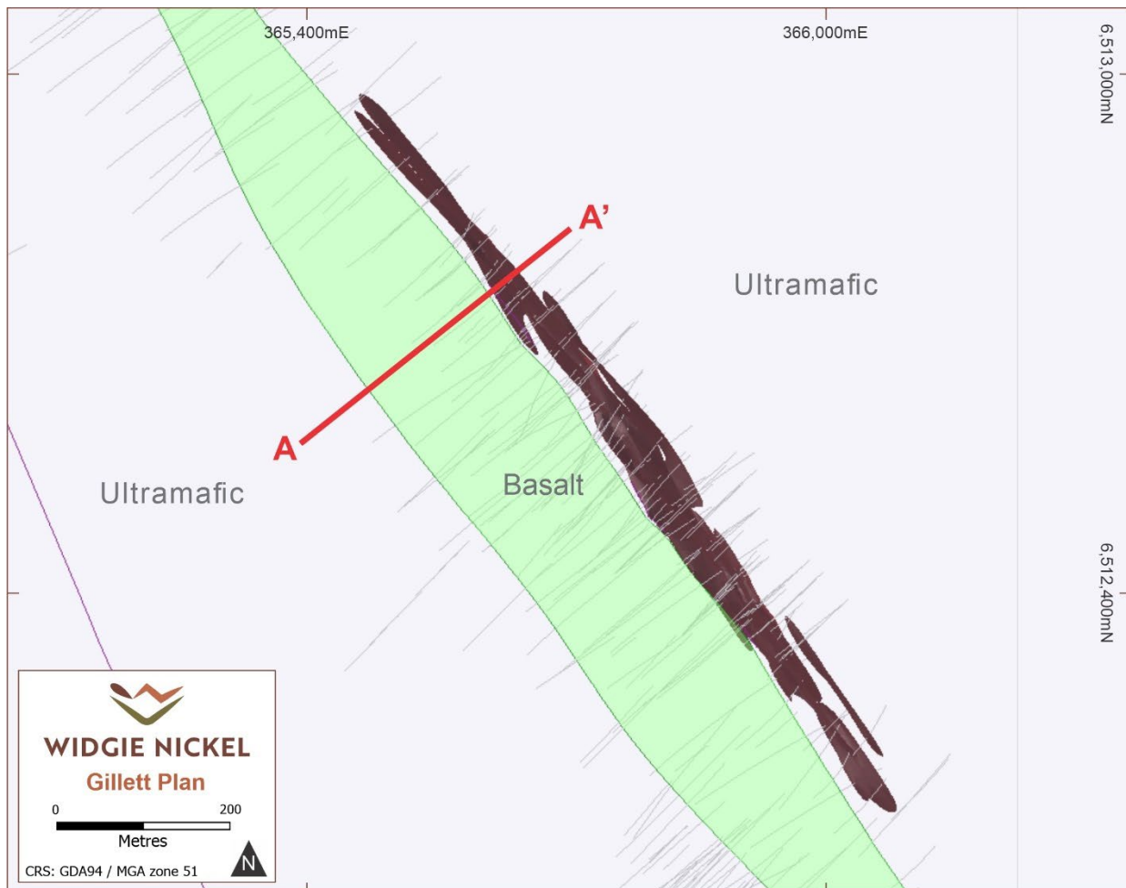
Figure 2 - Plan section showing the Gillett Mineral Resource envelope and the location of cross section A.
