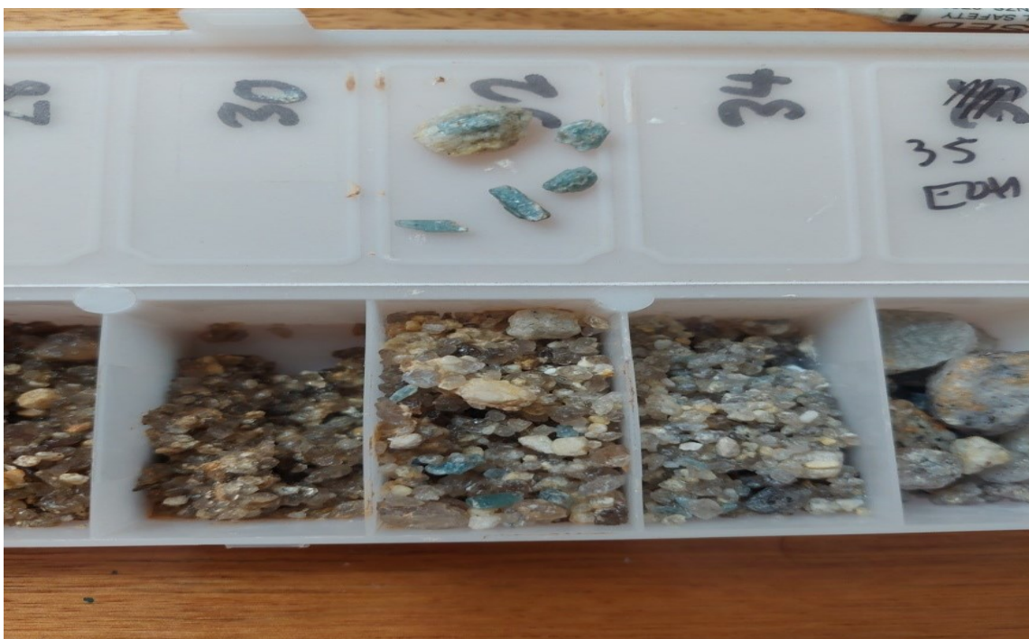
Figure 6. Chip tray showing the final 5m (30-35m) of hole 22DAC016. Downhole meterage is shown. The distinctive blue-green aqua marine is illustrated amongst the pegmatite chips.
