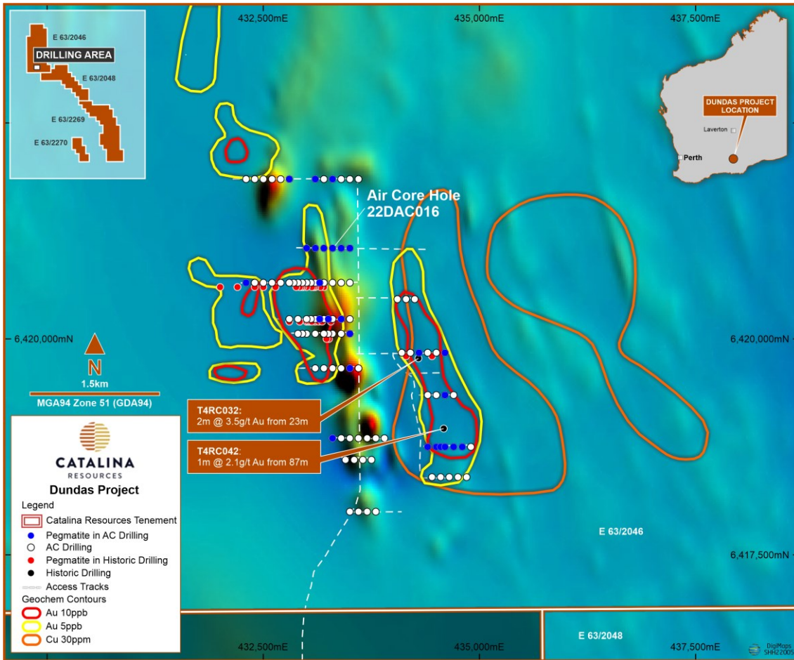
Figure 5. Air core drilling summary, location of hole 22DAC016 for southern portion of the tenement E63/2046. Underlying image is the regional aeromagnetic image.
