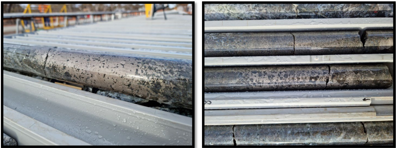
Photo 1: Ni-Cu sulphide mineralisation from OCDD001 from 545.2m and 579.5m at the Octagonal Prospect
