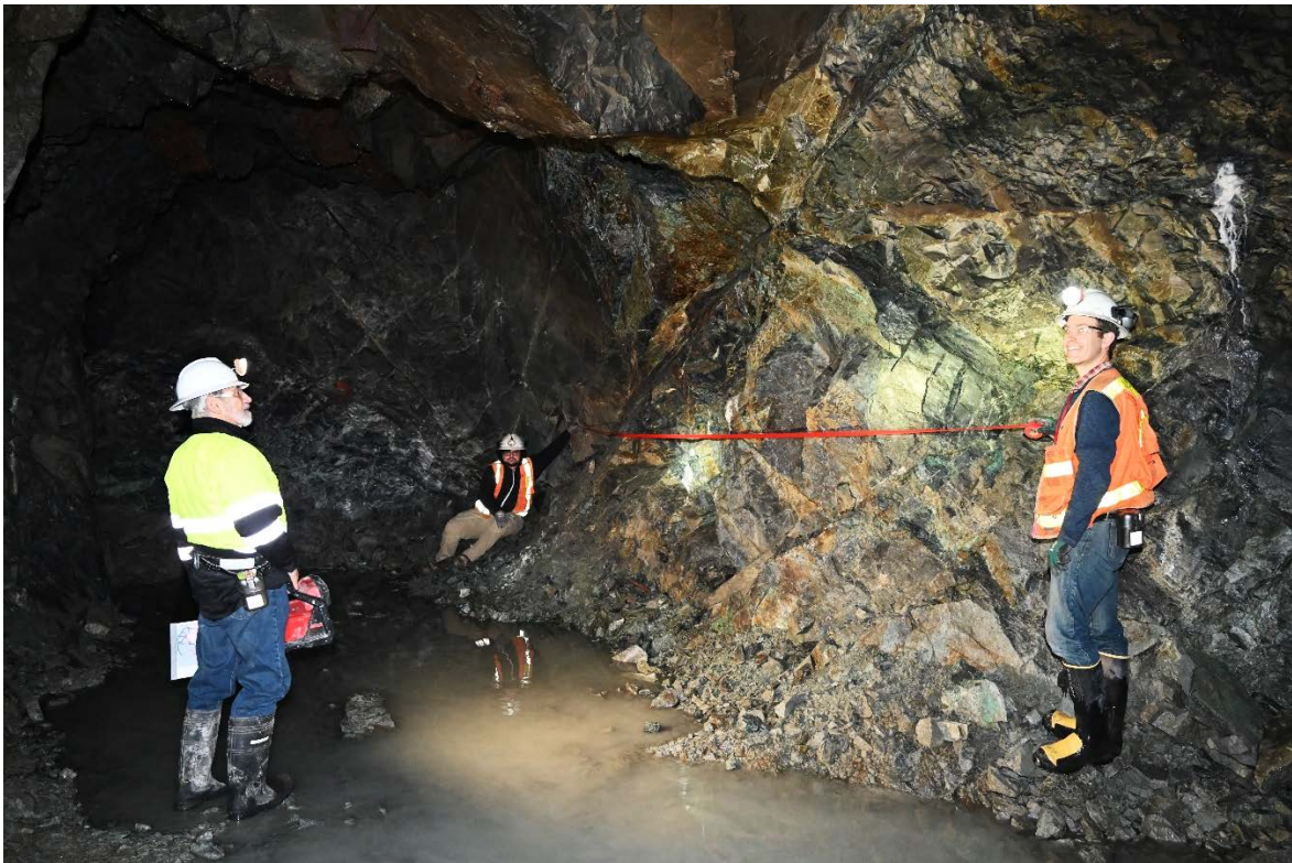
Photo 6 – Tape showing exposed mineralised zone in the Abrigo formation for planned channel sampling and mapping
