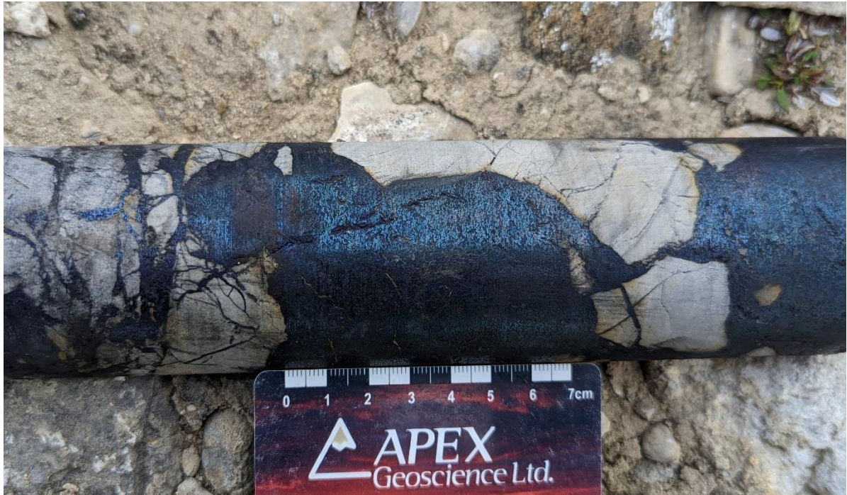
Figure 1: Massive bornite from approximately 50.9m downhole in 2022 drill hole ST22-05, which returned assays of 41m @ 4.18% Cu from 38m downhole.
