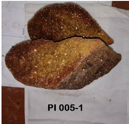
Figure 4 Sample PI 005-1 A highly micaceous rock which produced an assay grading 267.2ppm TREO and 1930ppm \text{Rb}_2\text{O}
