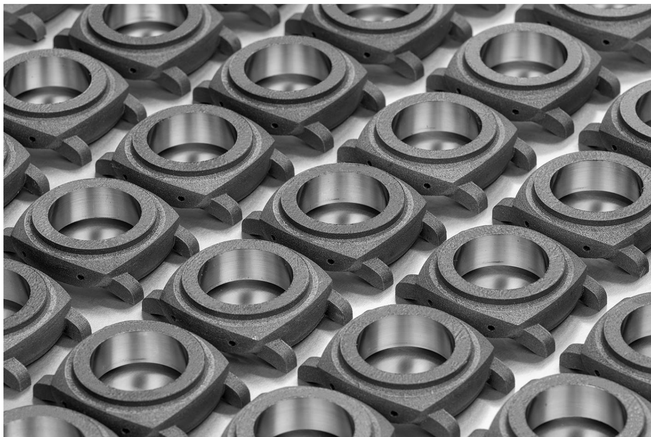
Figure 1: Panerai watch cases 3D printed using IperionX's low carbon, 100% recycled titanium powders.
