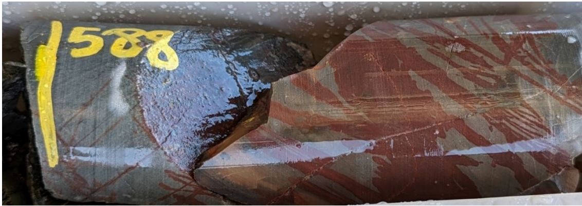
Figure 9 – ‘Bleed’ textured hematite alteration of siltstone (588m).
