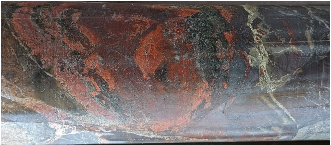
Figure 10 – Pyrite vein cutting hematitic ironstone (663.8m).
