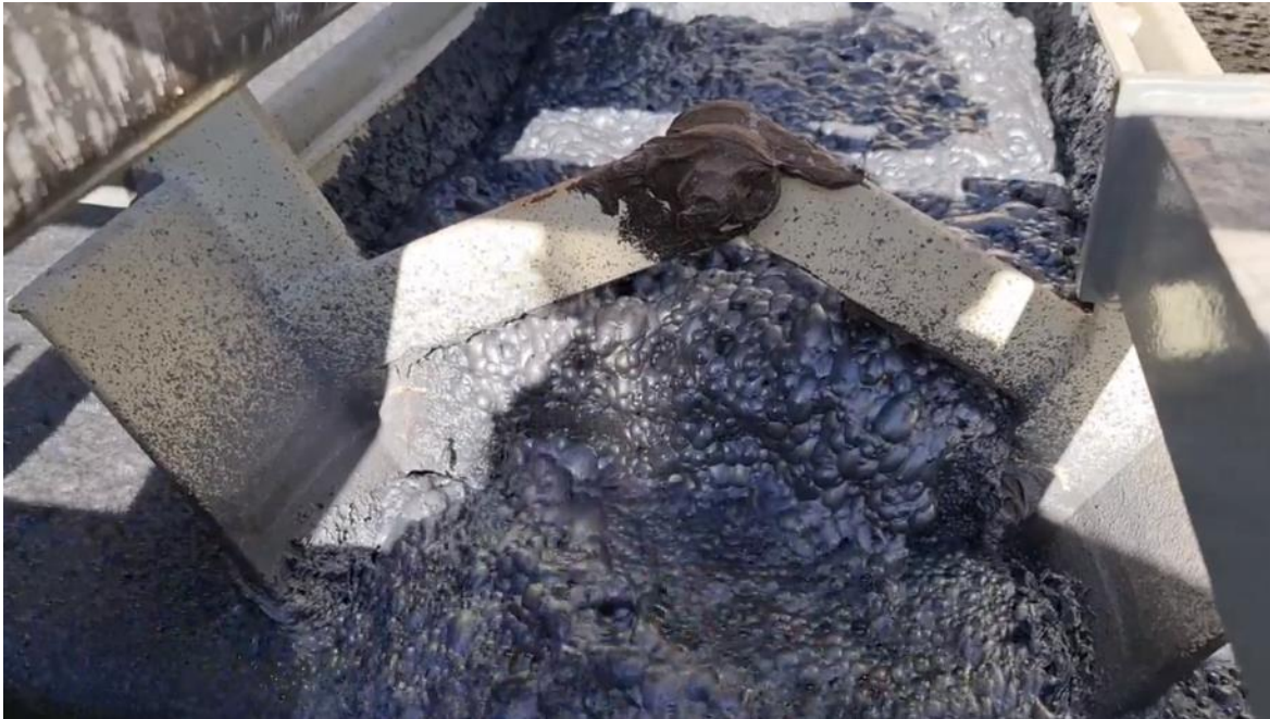
Figure 6 – High grade lead-silver concentrate in Abra's flotation tank (Photo 12 January 2023).
