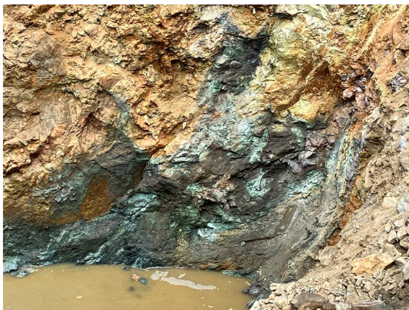
Figure 1: Massive sulphide Oxide Zone (yellow) to Transitional Zone (black) interface within the metallurgical slot during digging.
