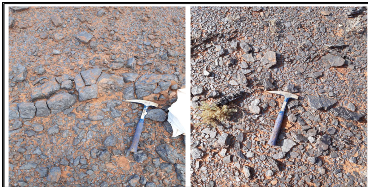
Figure 2 - Manganiferous shale samples within the Balfour Formation BR003 - 36.8% Mn (left) and BR008 - 28.9% Mn (right) from E52/4071
