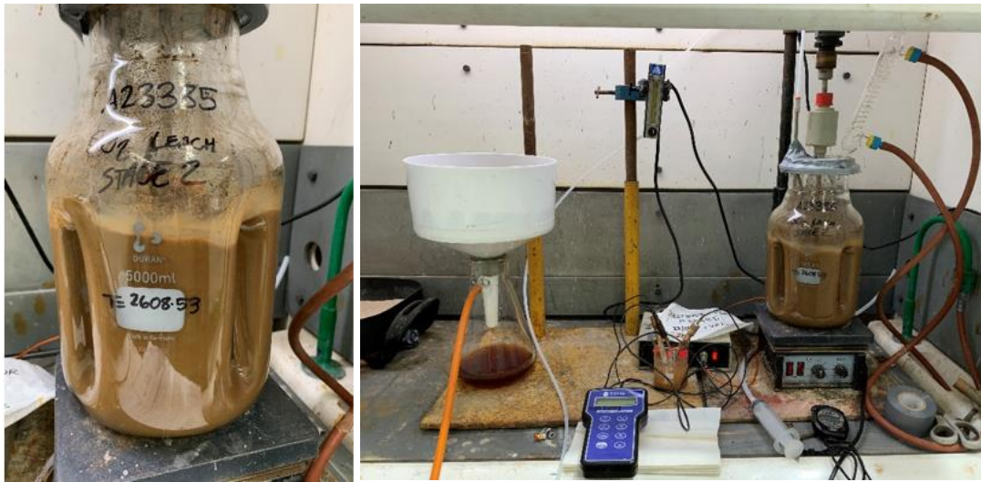
Figure 2: Leach Test (left) and test work setup (right)
