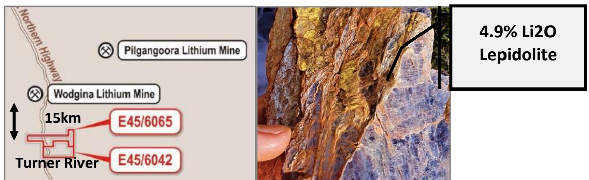
Figure 1: Location map of QXR's Turner River project mineral exploration licences relative to large Pilbara lithium mines, and photo of weathered lepidolite in rock samples from the drilling area shown in Figure 1.
