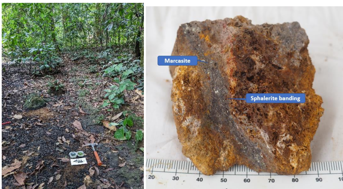
Figure 1: Newly discovered gossan and barite field (1.7km north of TP13) with sample R0125.
