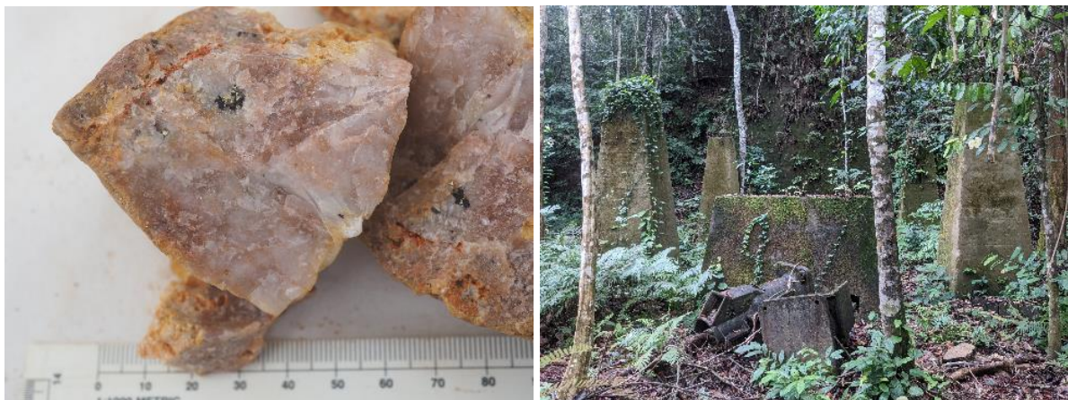
Figure 5: Quartz vein sample from Salane waste dump (R0177) – 30g/t Au (LHS) and historical processing plant footings (RHS)
