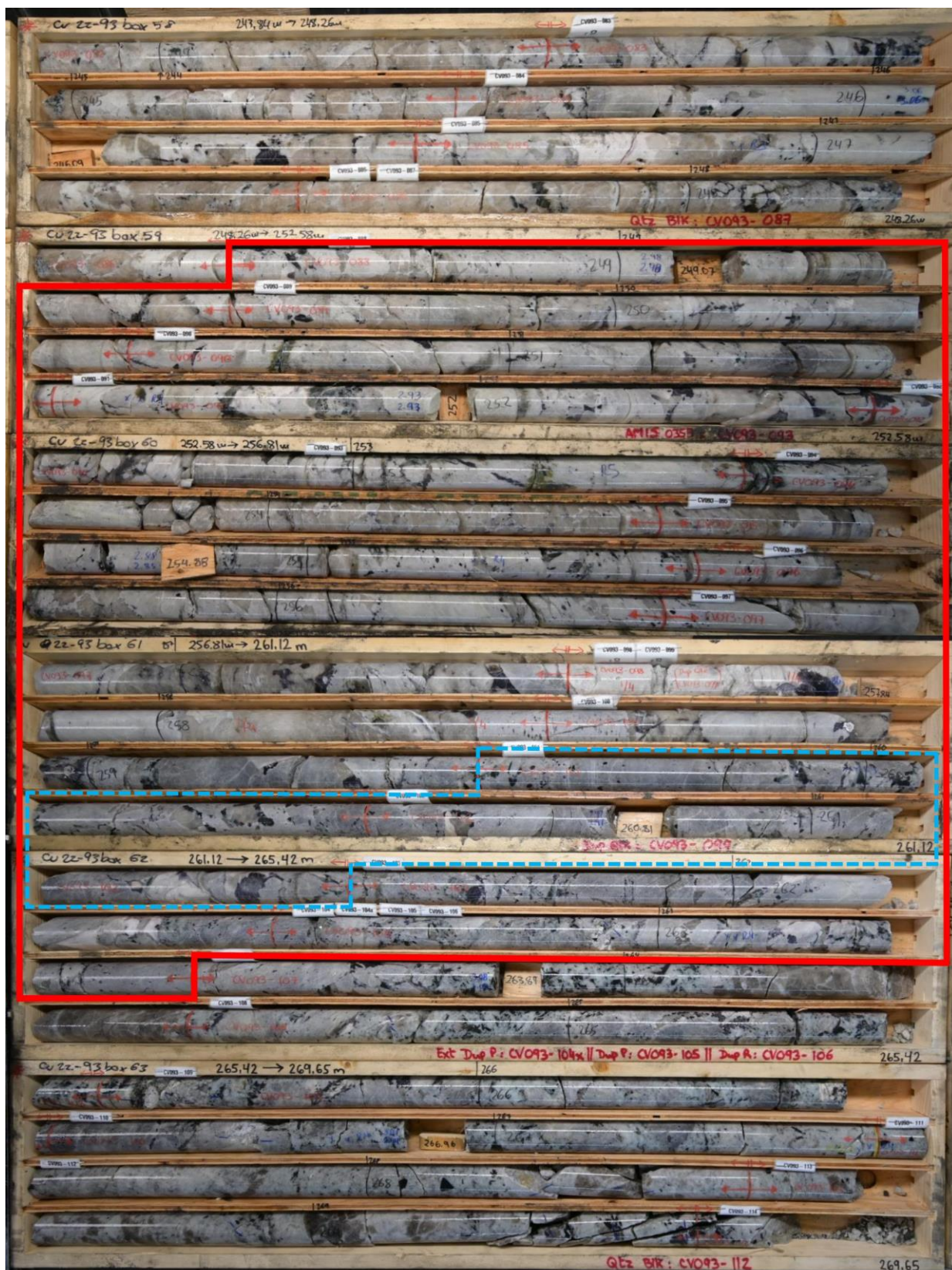
Figure 2: High-grade Nova Zone drill core intersection (15.0 m at 5.10% Li 2 O) in CV22-093 (red box), including 2.0 m at 6.17% Li 2 O (dashed blue box)
