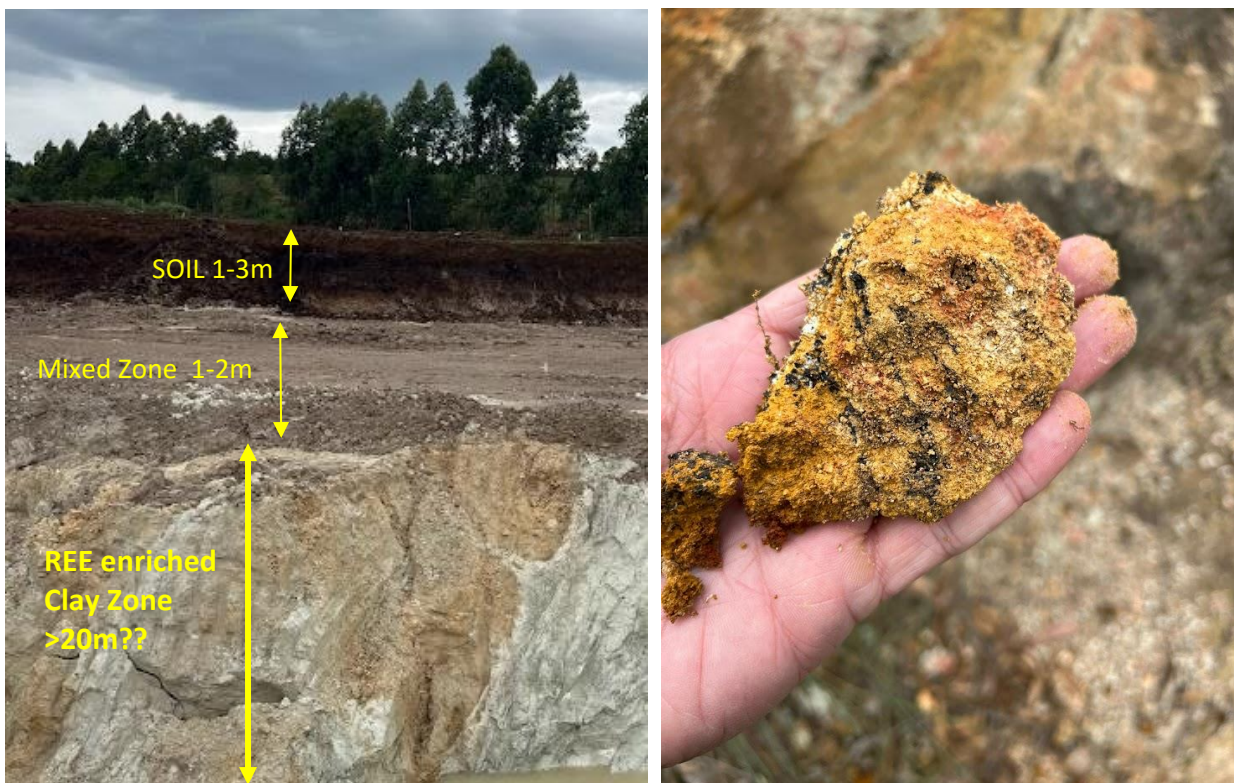
Figure 3. a) From Togni SA refractory clay mining pit at Capo do Mel (CDM) Project highlighting the thin soil horizon (approx. 1m this area). Mixed clay soil zone 1-2m thick and then the mineralised clay zone enriched in REE. b) Detail of REE enriched clay-zone sample from clay mining area on CDM Prospect. Note: the thicknesses of horizons may vary considerably across the project. REE mineralisation has been found in all zones.
