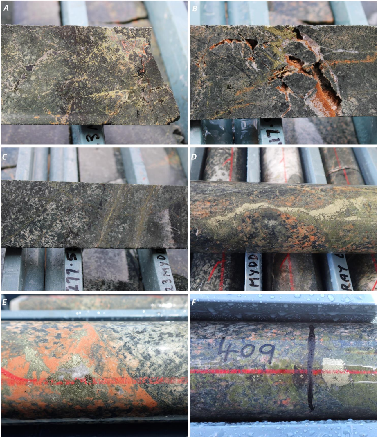
Figure 3. Images of various styles of mineralisation from the upper portion of hole 23MYDD422 (HQ drill core - 63.5mm diameter). A) Native copper (salmon pink, upper right) occurring with small patches of chalcocite (black/grey, centre left) from 161.8m; B) vuggy breccia zone partially infilled by chalcopyrite (yellow) and carbonate (white/orange) from 219.2m; C) chalcopyrite and pyrite veining/stockwork with epidote/chlorite selvedges in a strongly altered diorite host from 280.6m; D) brecciated, K feldspar-altered breccia zone with strong chalcopyrite-epidote matrix infill from 378m; E) brecciated diorite with chalcopyrite, pyrite and carbonate infill from 395m; F) strongly epidote-altered diorite with a large patch of chalcopyrite from 409m.
