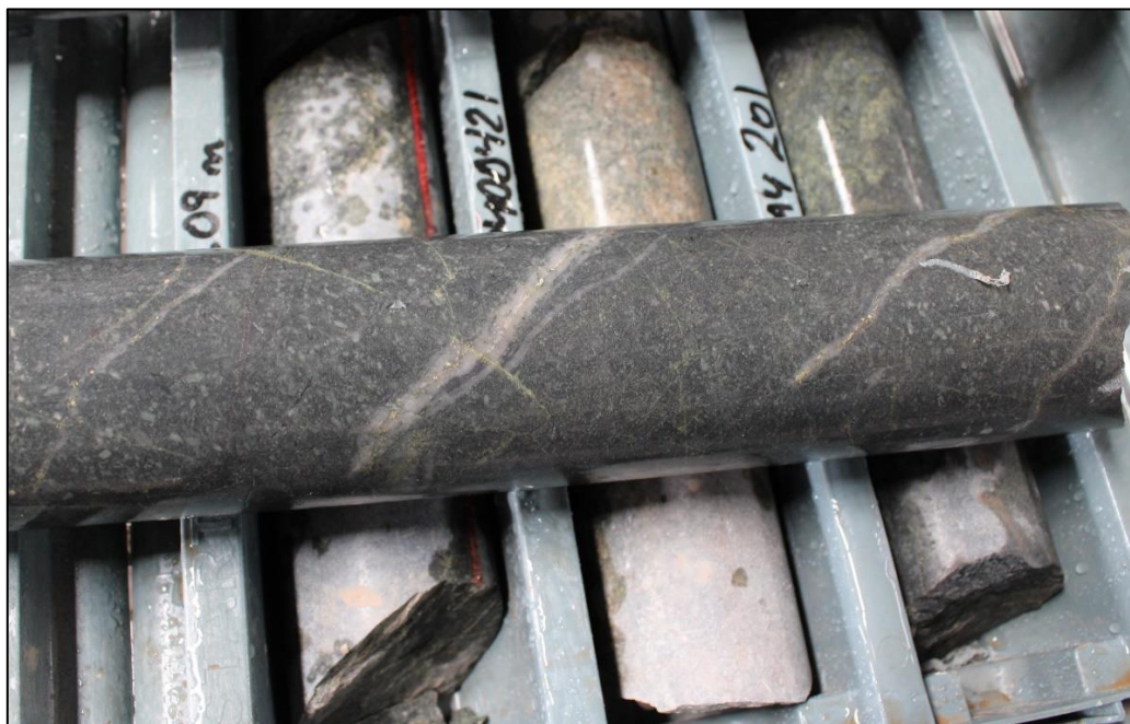
Figure 2. HQ diamond core from Corvette diamond hole 22MYDD421 at 817.5 metres, highlighting the abundance of early quartz veins with a centre-line of sulphides (also known as B-veins) crosscut by later epidote-chalcopyrite veins. This mineralisation forms part of a zone that grades 13 metres at 1.07% Cu & 0.61g/t Au.
