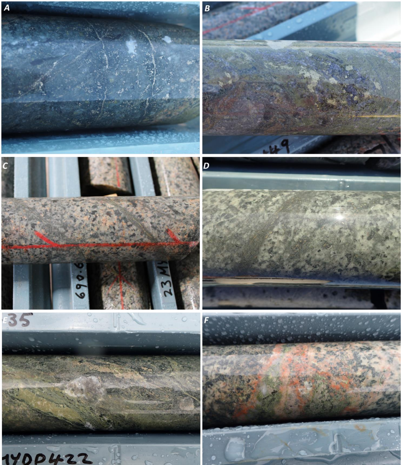
Figure 4. Images of various styles of mineralisation from the lower portion of hole 23MYDD422 (HQ drill core - 63.5mm diameter). A) Intense development of pyrite stockwork with lesser chalcopyrite in a strongly chlorite-altered porphyritic andesite from 560m; B) patchy chalcopyrite (yellow) and pyrite (brass colour) associated with a zone of intense epidote (green) alteration from 656m; C) fractured diorite hosting narrow sub-parallel pyrite/chalcopyrite veins with a chlorite selvage from 692.2m; D) disseminated and vein hosted pyrite with lesser chalcopyrite in diorite from 774.6m; E) strongly epidote/chlorite-altered andesite hosting elongate patches of pyrite and lesser chalcopyrite from 841m; F) fractured, hematite-dusted diorite hosting quartz-epidote-pyrite-chalcopyrite infill from 1,066m.
