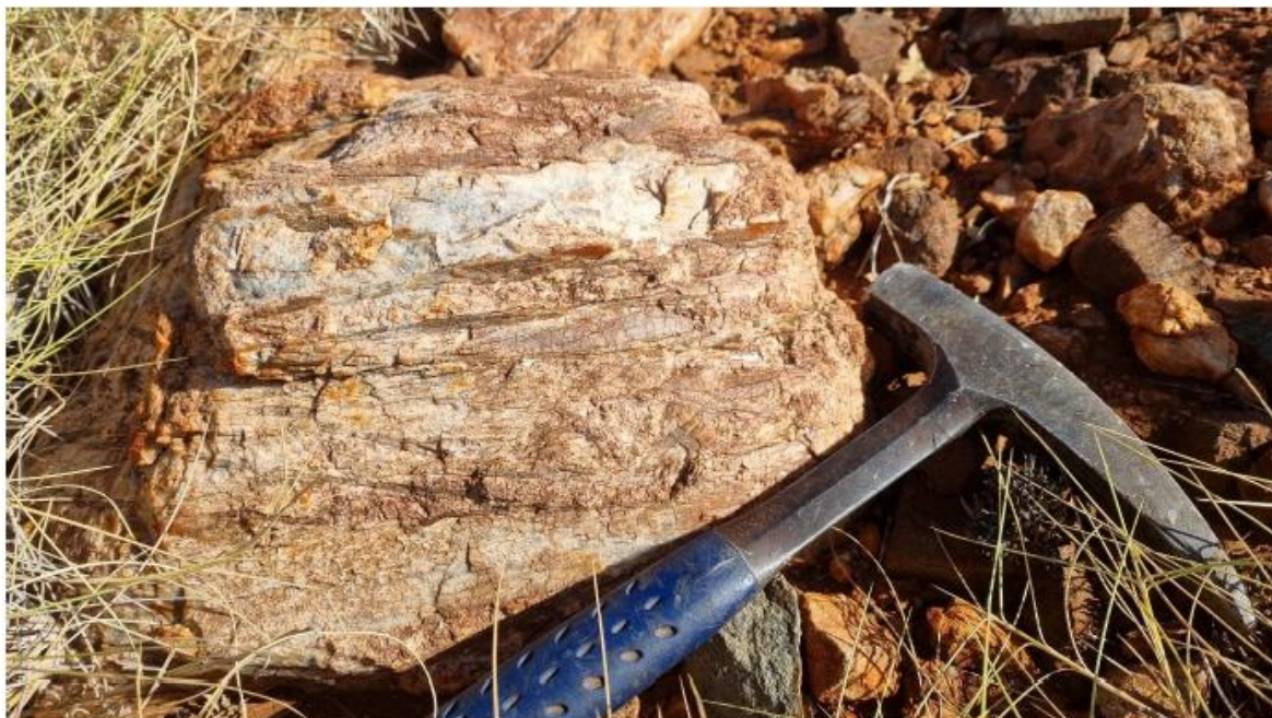
Image 1: Spodumene-rich pegmatite at AP0006 (see Figure 2) associated with samples APRK00867 (4.39% Li 2 O), APRK00870 (4.31% Li 2 O), APRK00872 (4.28% Li 2 O) and APRK00874 (4.41% Li 2 O)
