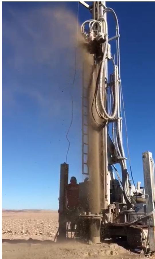
Figure 3: High pressure brine encountered in drilling
