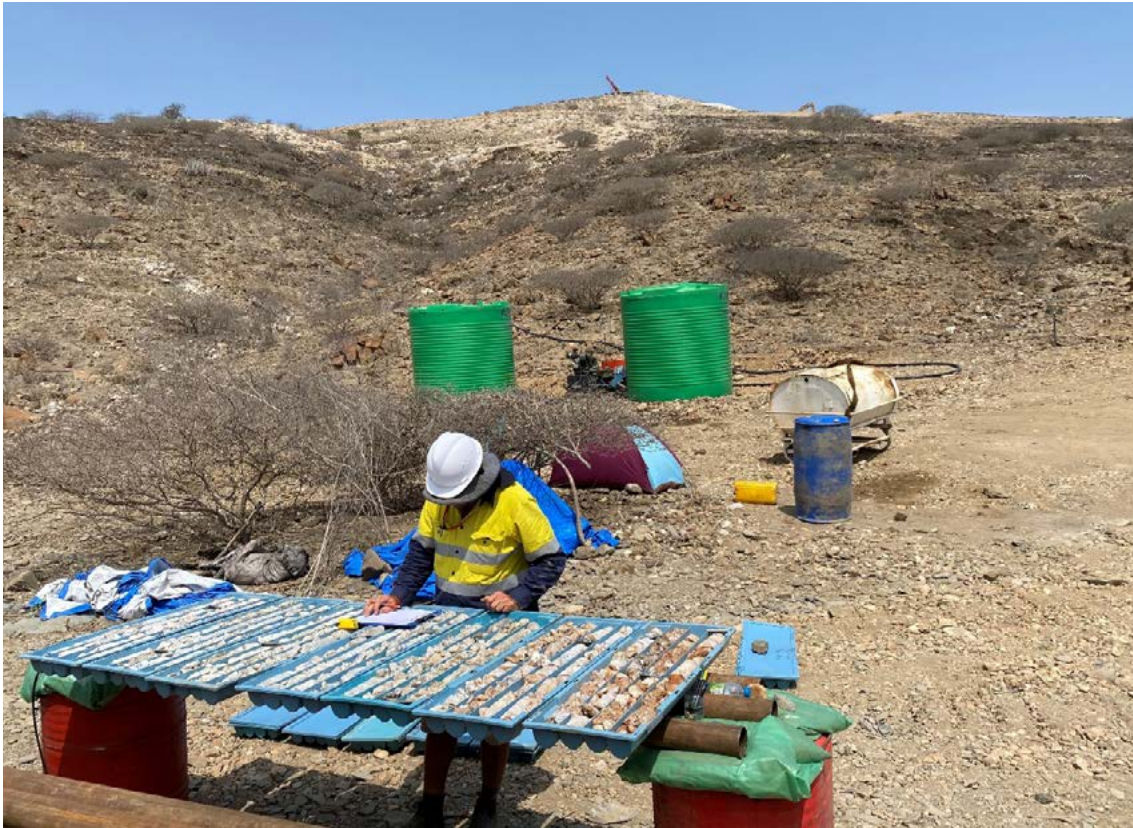
Figure 3: Core-trays laid-out on makeshift core rack at site. Note drill-rig in background on top of hill, set-up on drill-hole NDDH004. Geologist Neil Scholtz logging drill-core from NDDH004
