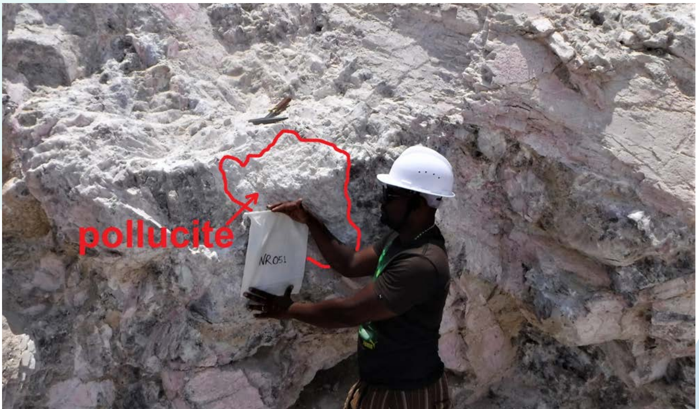
Figure 8: Exposed pollucite mass sampled as NR051. Field and logistics assistant Joao Paulo Boy provides scale
